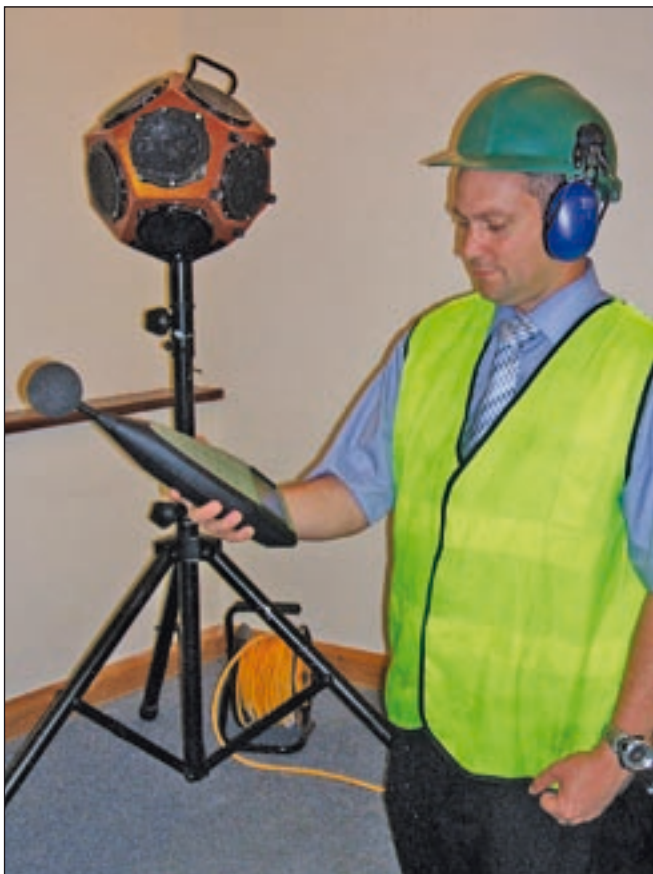
Acoustic testing on site (photograph courtesy of Sound Research Laboratories Ltd)
